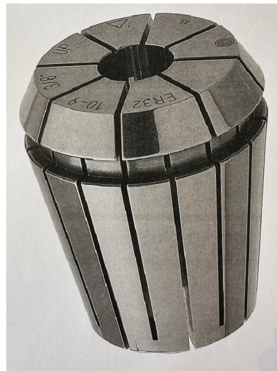
Single ER collet — precision-ground clamping surface
